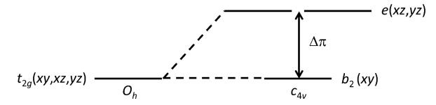
The  $d\pi$ -orbital splitting for a tetragonal oxo- or nitrido-metal complex is shown above.
